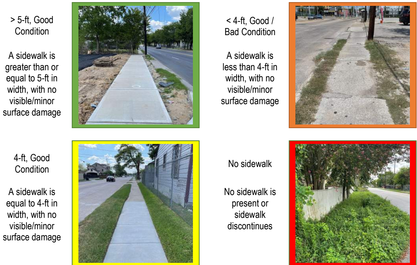
Figure 3.1. Sidewalk Assessment Definitions
