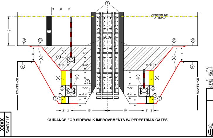
NOTES: 1. THE PURPOSE OF THIS DOCUMENT IS TO PROVIDE THE DESIGN ENGINEER WITH THE GUIDELINES FOR SIDEWALK IMPROVEMENTS W/ GATE ARMS AND EMERGENCY EXIT ROUTES.
